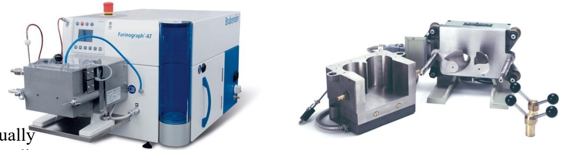
Fig.1.FARINOGRAPH®-AT and work camera
